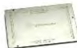
Calibration plate Bruker, 5023-0208
